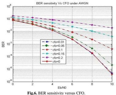
Fig.6 shows that the performance of OFDM will degrade with increasing the ratio of the maximum frequency offset to carrier spacing (i.e. CFO). The system can maintain the performance in the presence of smaller CFO. It is seen from figure.6 that increase in SNR( Eb/No) reduces Bit error rate. Now the value of CFO is varied from 0 to 0.3 keeping rest of the parameters same. It is seen from fig.7 that the performance still degrades and the curve shows a flat response.
