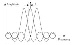
Fig.2. Inter-carrier interference(ICI)
