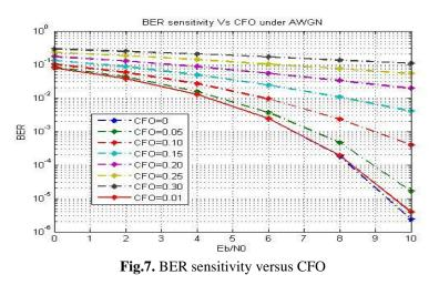
The degradation of SNR, Dfreq, caused by the frequency offset is approximated by the equation  $D_{freq} \cong \frac{10}{3\ln 10} (\pi \Delta fT)^2 \frac{E_b}{N_0}$
