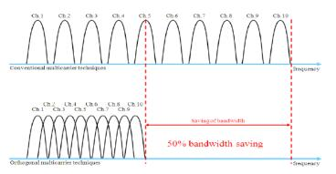
**Fig.1.** Bandwidth saving in OFDM
