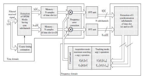
Fig.3.CFO synchronization using pilot tones
