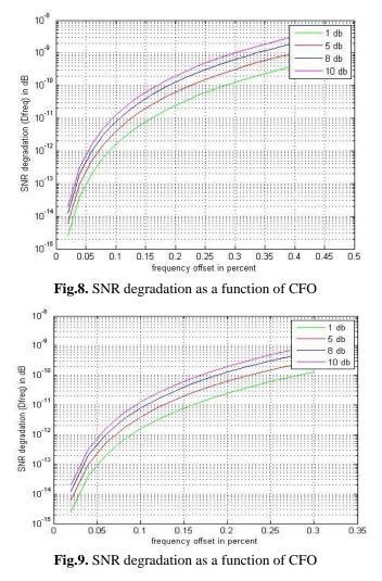
The OFDM system parameters are CFO = 0.15 and, N = 128, Ng = 16,Nps = 4 (Pilot spacing), Number of pilots Np = 32, signal to noise ratio (SNR) 0 to 25 dB , D is an integer. D=1,2,4, For OFDM mapping, QAM modulation is used. Signal energy Es = 1.
