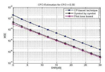
Fig.5. Comparision between CFO estimation methods.
